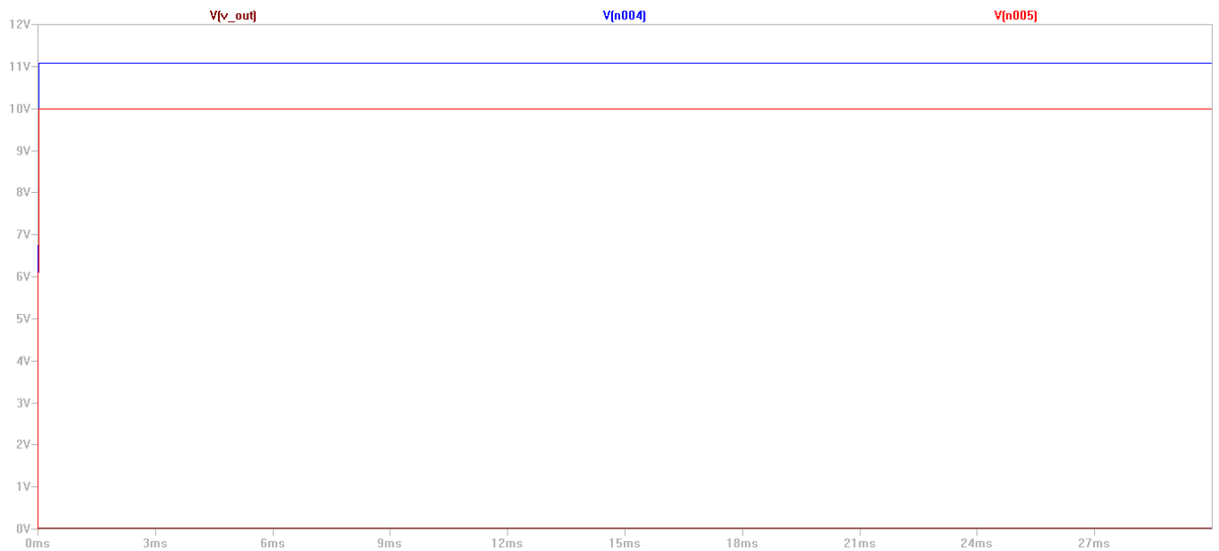
Figure 4-14: Output Voltage of LT1716 when Battery Level is Below 11V and Requires Charging
