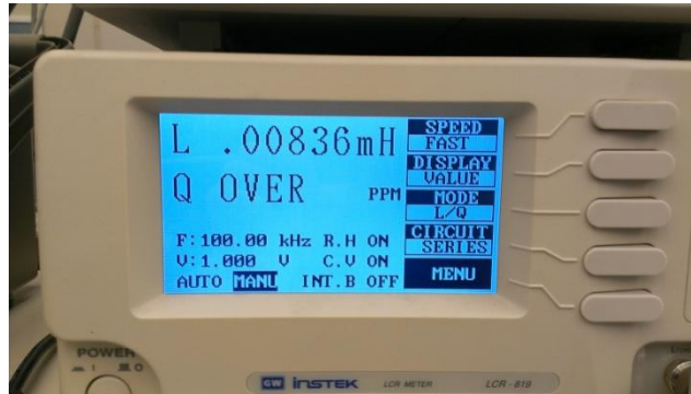
Figure 5-2: Primary Inductance Value of Flyback Transformer at 100 kHz
