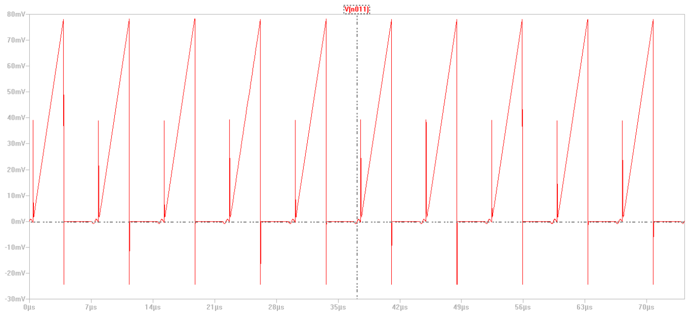
Figure 4-5: Simulated Voltage at Sense Pin at Full Load (2A) for Charging Flyback
