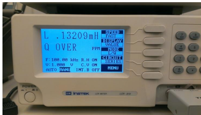
Figure 5-3: Secondary Inductance Value of Flyback Transformer at 100 kHz
