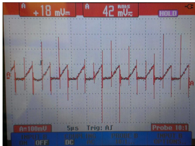
Figure 5-10: Current Sense Voltage of the Sense Resistor for the Charging Flyback and Output Voltage Peak-to-Peak Ripple at Full Load Conditions
